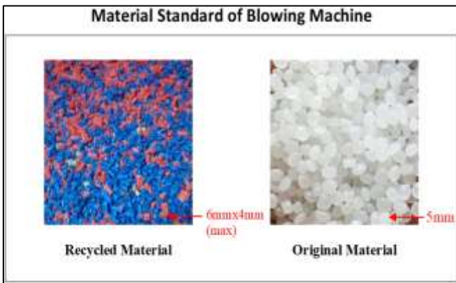
Figure 6. Material standard of blowing machine
