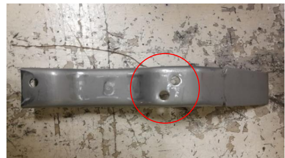
Fig. 1. Sliding hole defects
