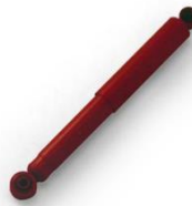
Gambar IV. 7 Shock Breaker Oil Type Damper
