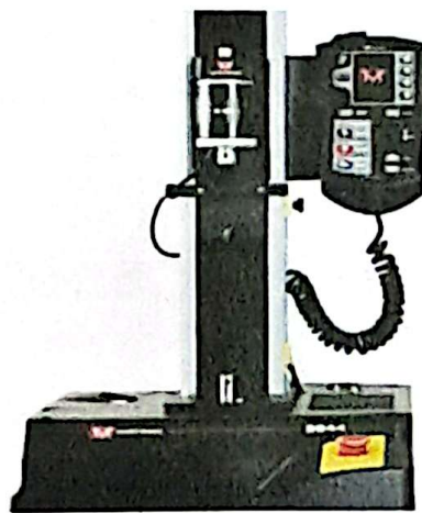
Gambar 2.7. Universal Testing Machine (UTM) Compressive Test
