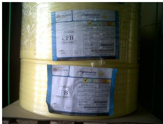
Gambar IV.5 kertas Carbonless CFB (Coated Front and Back) Lembar Tengah Sumber : PT. PDPPM (2015)
