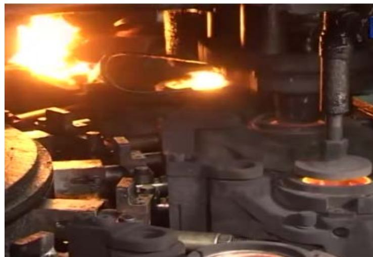
Gambar 4.8 Pencetakan gelas (Sumber: PT The First National Glassware )
