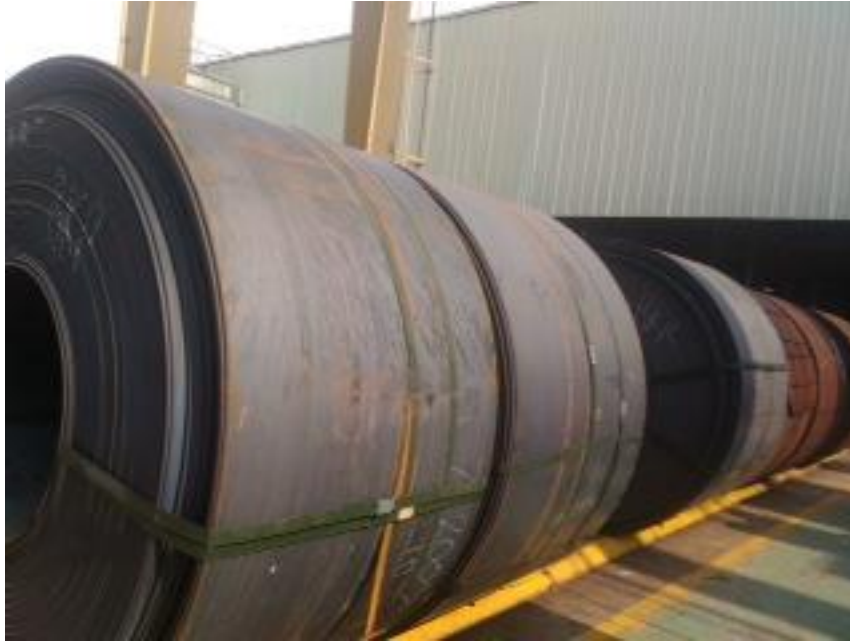
Gambar 4.3 Hot Rolled Coil ketebalan 6 mm.
