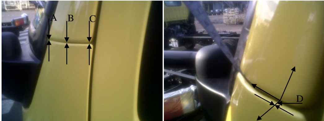
Gambar 4.7. Point-Point Pengukuran Corner Panel Terhadap Pillar Sumber: PT Krama Yudha Ratu Motor, 2013
