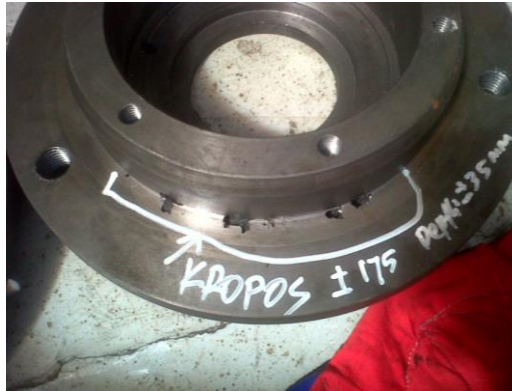
Gambar 5.1 Cacat Kropos Pada Komponen Housing Wrist Pin (Sumber : Divisi Oil and Gas Equipment )
