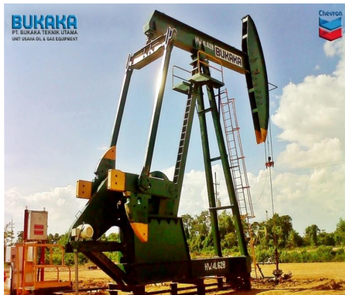
Gambar 4.1 Produk Pumping Unit PT Bukaka Teknik Utama (Sumber : Divisi Oil and Gas Equipment )
