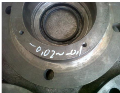
Gambar 5.2 Defect Lubang Bearing (Tirus) Pada Komponen Housing Wrist Pin (Sumber : Divisi Oil and Gas Equipment )
