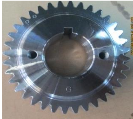
Gambar 4.7 Gear crank TF 135 (Sumber: PT Morita Tjokro Gearindo, 2016)
