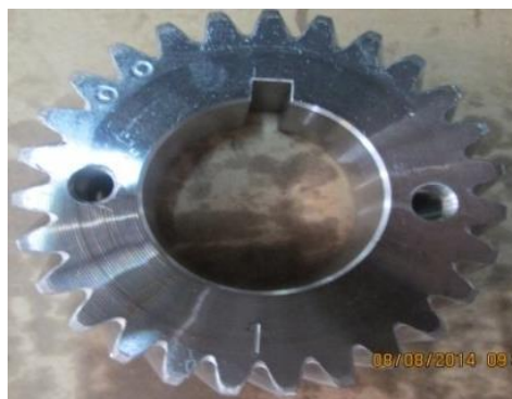
Gambar 4.3 Gear crank RD 75 (Sumber: PT Morita Tjokro Gearindo, 2016)
