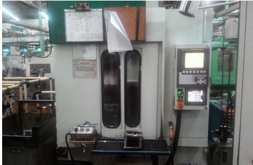
Gambar 4.9 Mesin shaving type GSF-400B-NC3 (Sumber: PT Morita Tjokro Gearindo, 2016)
