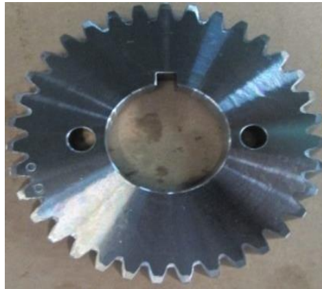
Gambar 4.5 Gear balancer drive TF 105 (Sumber: PT Morita Tjokro Gearindo, 2016)
