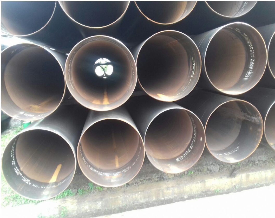
Gambar 4.3. Pipa Baja Standar ASTM A53 di Plant KT 24 PT BIP
