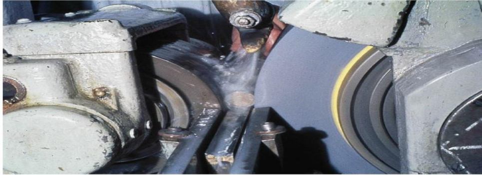
Gambar IV.8 Skema Proses Face & Outside Dimension Grinding (Sumber : PT SKF Indonesia)
