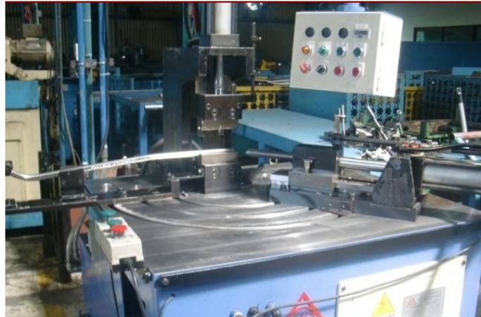
Gambar 4.10 Proses Notching Pipe (Sumber: PT Pamindo Tiga T)
