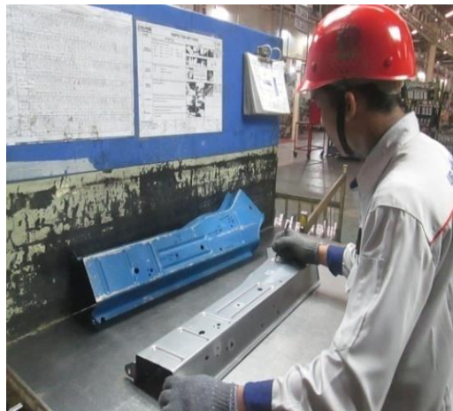
Gambar 4.9 Proses Final inspection (Sumber: PT Mekar Armada Jaya)
