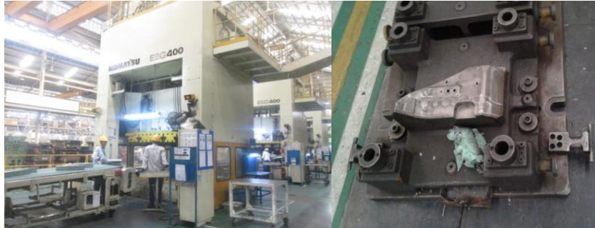
Gambar 4.7 Proses Bending dan Dies Proses Bending
