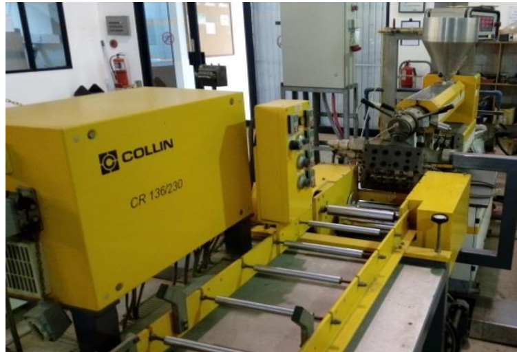
Mesin Ekstruder Single Screw dan Callendering
