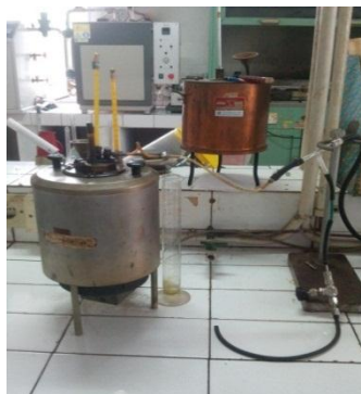
Gambar 3.2 Alat Uji Flash Point “ABEL”
