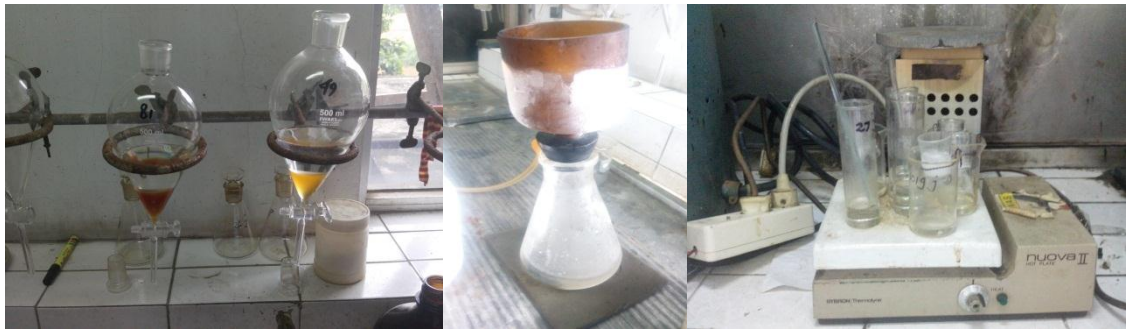
Gambar 3.5 Alat Uji Wax Content
