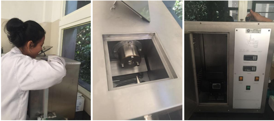
Gambar C.6 Proses Uji Water Washout
