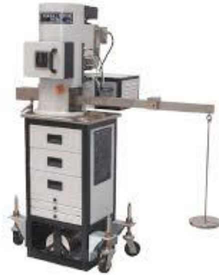
Gambar III.5 Alat uji four ball
