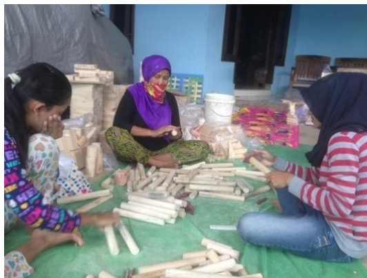
Gambar 4.13. Proses Pengamplasan Manual
