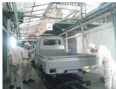
Gambar 4.6. Proses Sanding (Sumber : PT Krama Yudha Ratu Motor)
