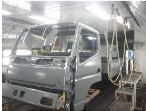
Gambar 4.7. Proses Sealing dan Under Coat (Sumber : PT Krama Yudha Ratu Motor)
