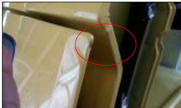
Gambar 4.17. Jenis cacat Ex-Repair (Sumber : PT Krama Yudha Ratu Mootr)
