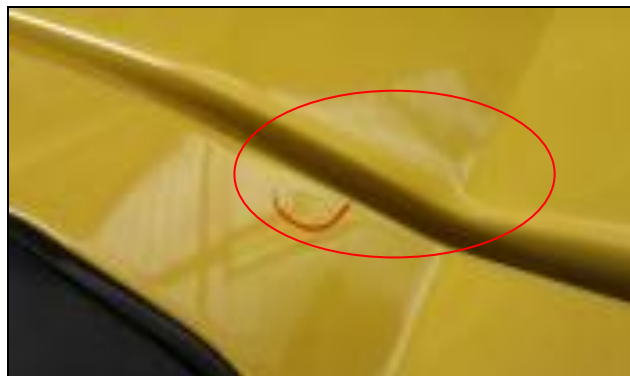
Gambar 4.15. Jenis cacat Sagging (meleleh) (Sumber : PT Krama Yudha Ratu Motor)
