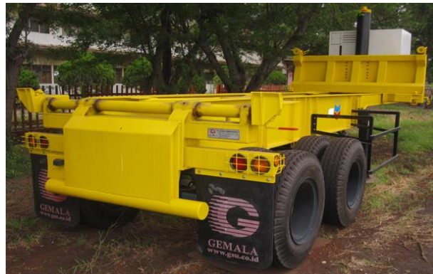
Gambar IV.16 Tipping Trailer (Sumber: PT Gemala Saranaupaya, 2017)
