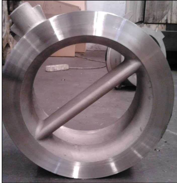
Gambar IV.8 Swing Wafer Check Valve (Sumber: PT Samudera Berlian Metalindo, 2015)
