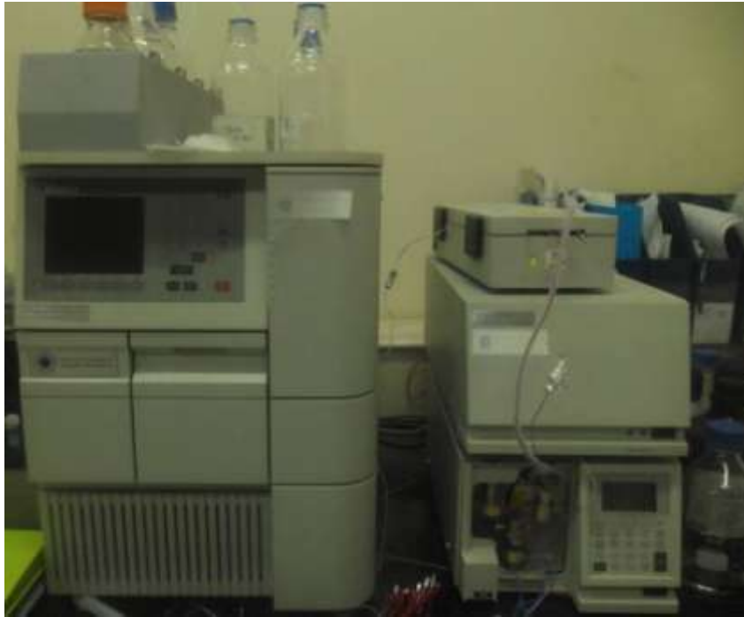
Gambar 3. Instrumen HPLC Waters Alliance Tipe e-2695
