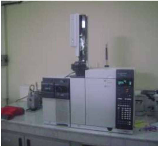
(a) Gass Chromatography Mass Spectrum (GC-MS) Agilent type 15977A Series.
