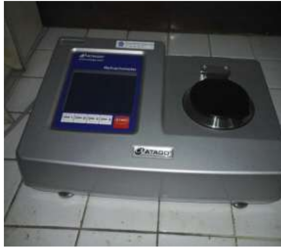
(b) Refraktometer digital RX-5000a 150528N Atago
