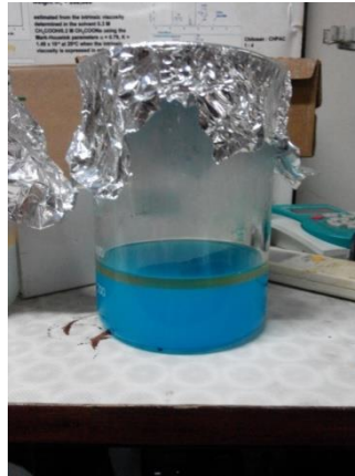
Gambar 4.2 Polystyrene-co-acrylic acid (B) 1 mol styrene , 1 mol acrylic acid dan \text{CuSO}_4
