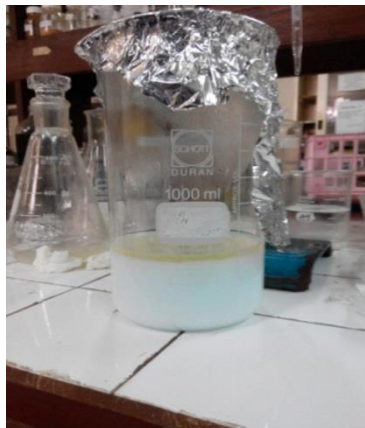
Gambar 4.1 Polystyrene-co-acrylic acid (A) 1 mol styrene , 1 mol acrylic acid
