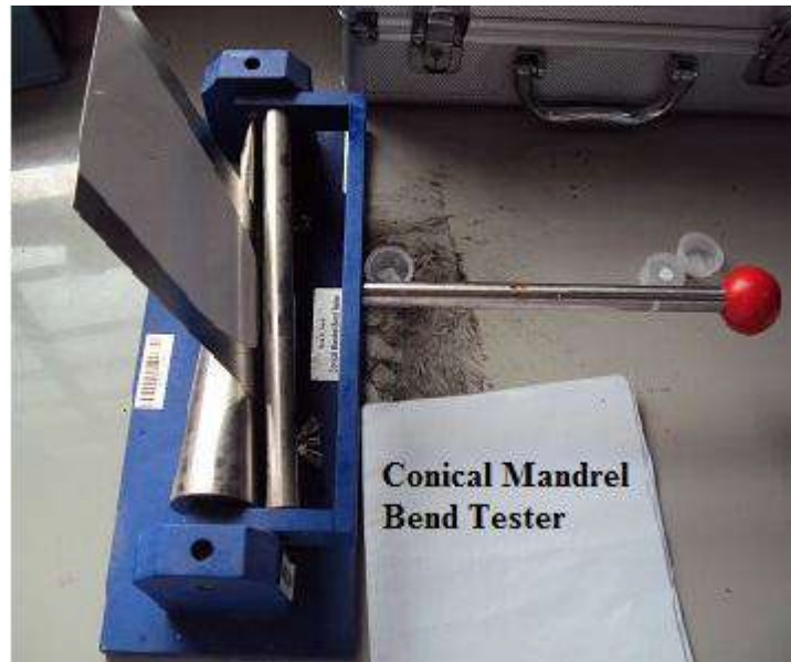
Gambar 9. Alat Conical Mandrel Tester
