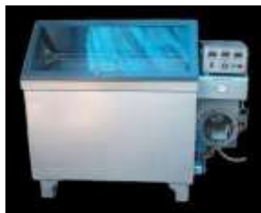
Salt Spray Cabinet
