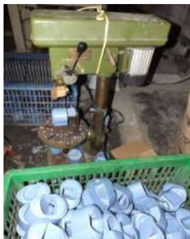
Gambar 4.8 Proses Pengeboran onion Slicer Destec
