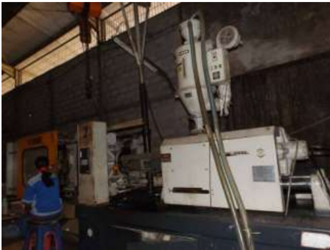
Gambar 4.7 proses pencetakan body, receiver dan handle onion slicer
