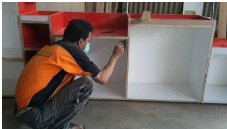
Gambar IV.21 Menyusun bagian-bagian kitchen set
