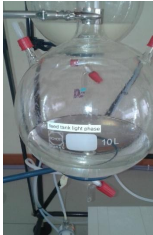
Gambar 3.5 Tabung Feed Tank Light Phase berisi Etanol 96%
