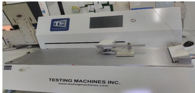
Gambar 3.1 Alat Uji Coefficient Of Friction (CoF)
