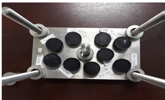
Gambar 5 Sampel Uji Mekanis Compression Set
