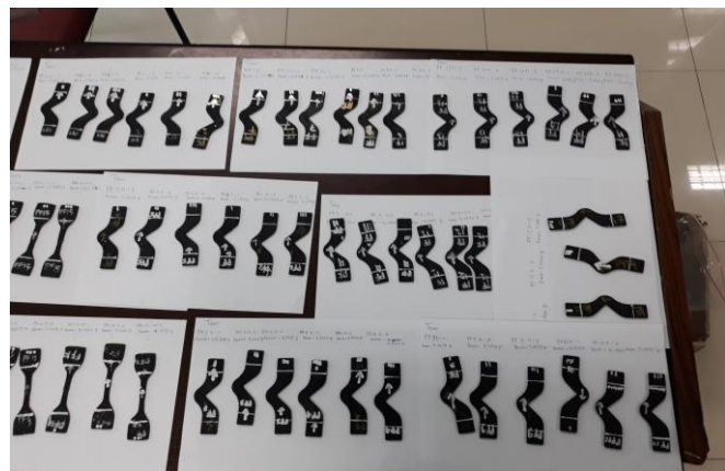
Gambar 4 Sampel Uji Mekanis Tear Strength
