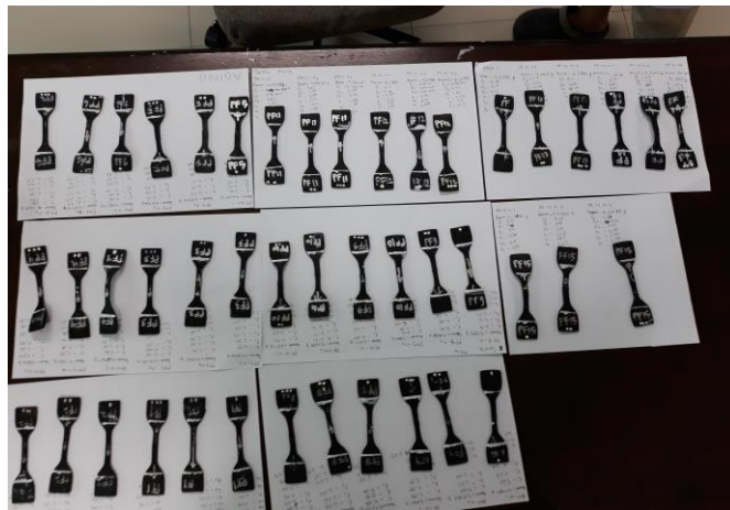
Gambar 3. Sampel Uji Mekanis Tensile Strength dan Elongation At Break
