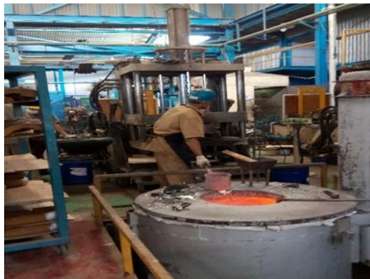
Gambar 4.10 Tungku Holding (Sumber: PT XYZ, 2017)
