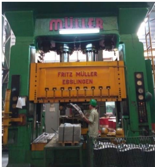
Gambar 4.14 Mesin PM 02 Hydraulic Power Press (400 Ton) (Sumber: PT Cidas Supra Metalindo)
