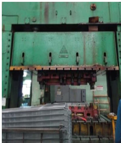
Gambar 4.13 Mesin PM 01 Hydraulic Power Press (1500 Ton) (Sumber: PT Cidas Supra Metalindo)
