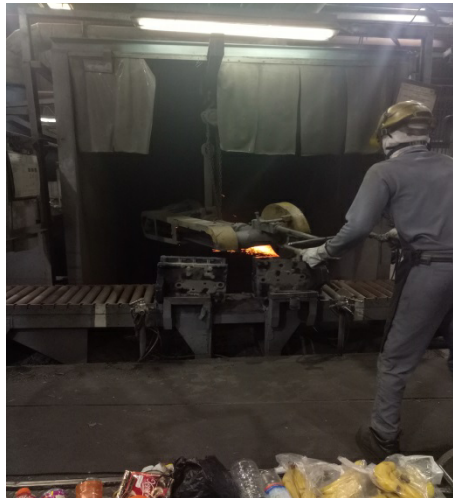
Gambar 5.6 Proses Gerinda Line Finishing
