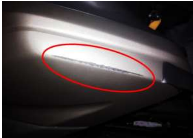
Gambar 4.9 Defect Scratch (Goresan) (Sumber : PT Sugity Creatives)
