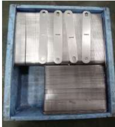
Gambar 4. 11 Hasil Blank-Piercing Clamp Piping JK-246760-0290 (Sumber: PT Hadeka Primantara)
