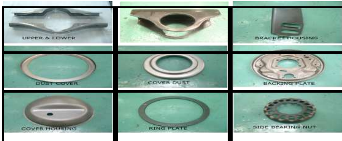
Gambar 4.4 Produk Pressed Parts (Housing, Bracket, Dust cover, Backing Plate, Ring Plate dan Side Bearing Nut)
