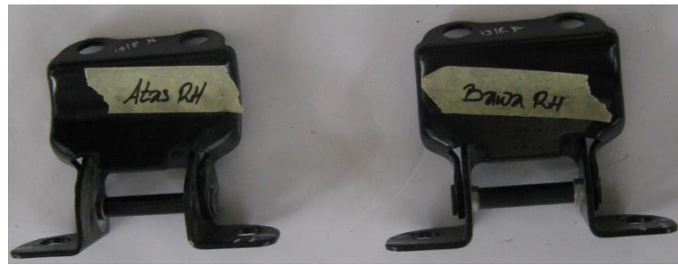
Gambar 4.4 Part Rear Door Hinge (Sumber: IOI)
