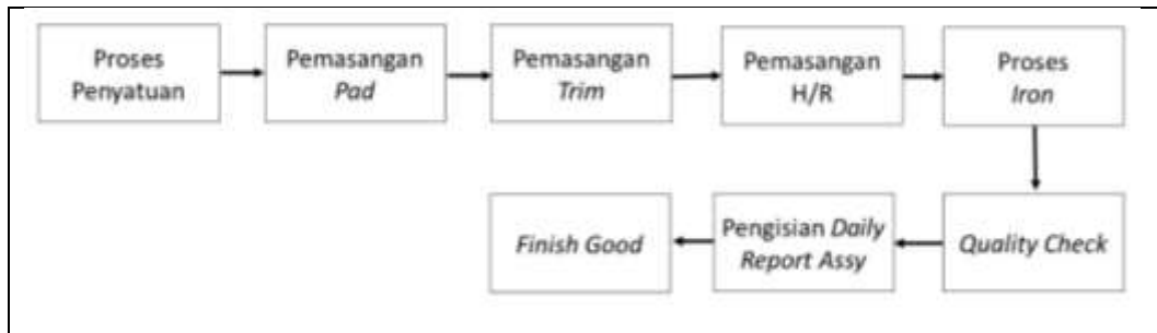
Gambar IV.5 Alur Proses Assembling Seat (Sumber: PT Suzuki Indomobil Motor Cikarang Plant, 2017)
