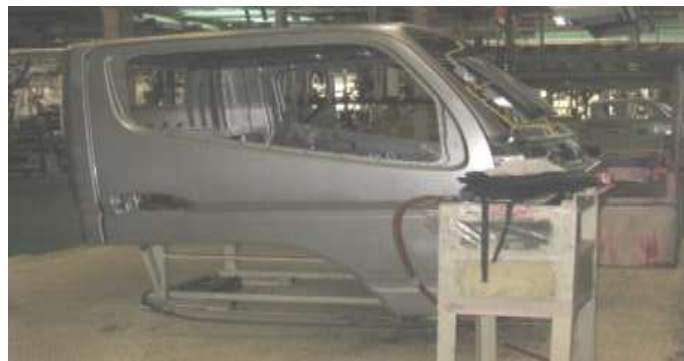
Gambar IV.27 Proses Down Door Install (Sumber: PT
