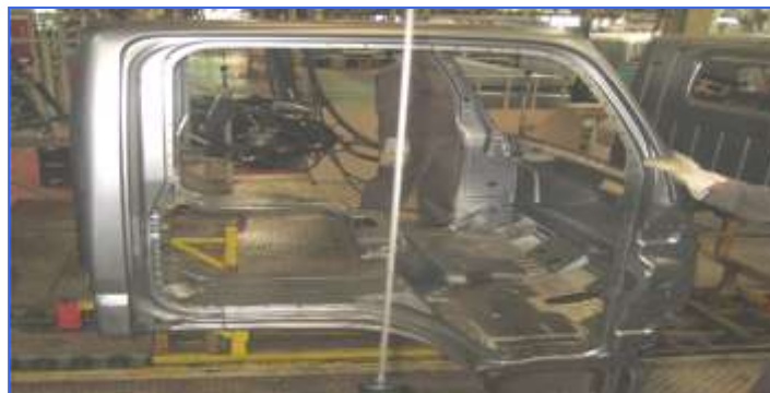
Gambar IV.25 Proses Main Body Respot 2 (Sumber: PT
