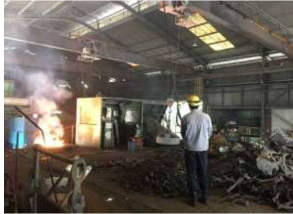
Gambar 4.17 Proses Pre-Charging Sumber: PT Bakrie Autoparts
