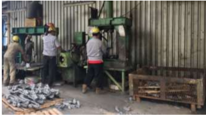
Gambar 4.22 Proses Fettling Sumber: PT Bakrie Autoparts
