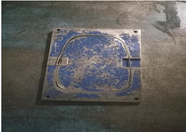
Gambar 4.8 Jig Inspection Wire Sifting Hole D01N
