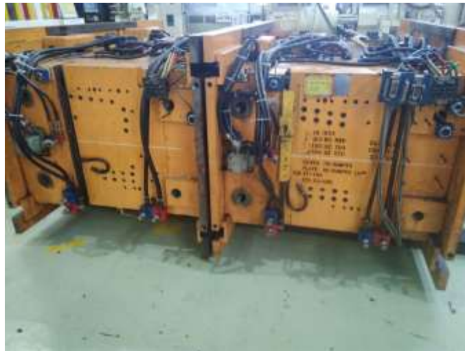
Gambar 4.3 Alat Pencetak Front Bumper
