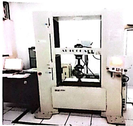
Gambar III. 2 Alat Uji Universal Testing Machine (UTM) Sumber: Pusat Penelitian Biomaterial LIPI, Cibinong
