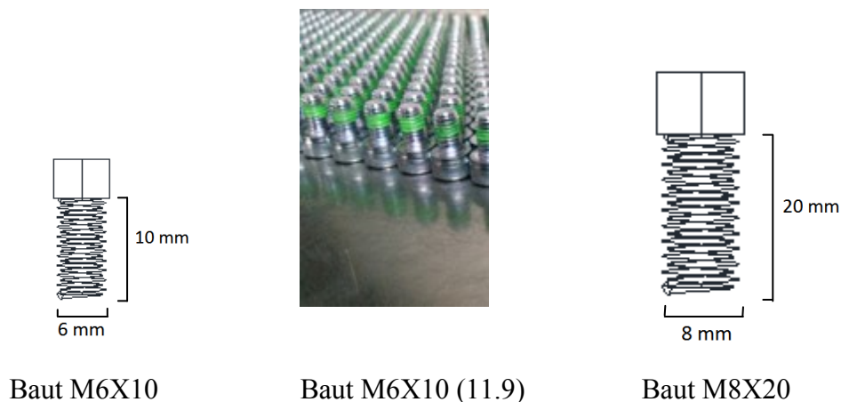
Gambar 4.3 Coating Bolts M6X10, M6X10(11.9), M8X20 (Sumber: Dokumen PT STAHL ARBEIT)
