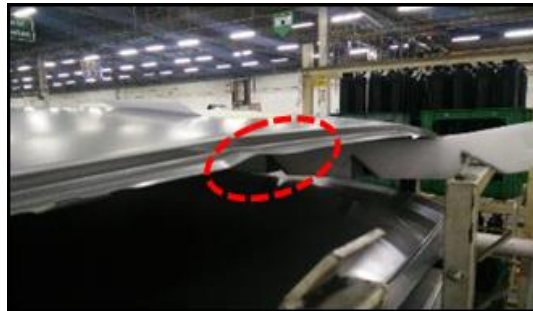
Gambar 4.11 Defect Deform Part Panel Roof (Sumber: PT TMMIN)
