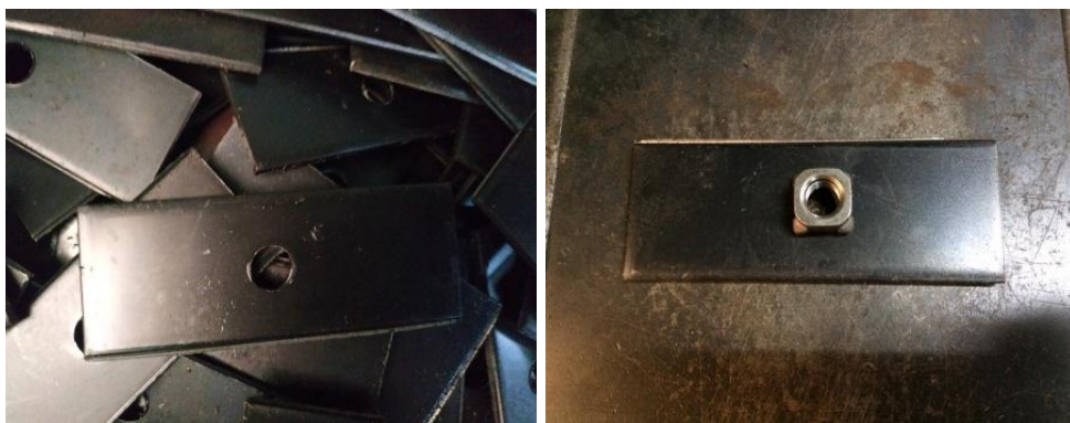
Gambar 4.9. Part Dudukan Baut Tank Comp Fuel
