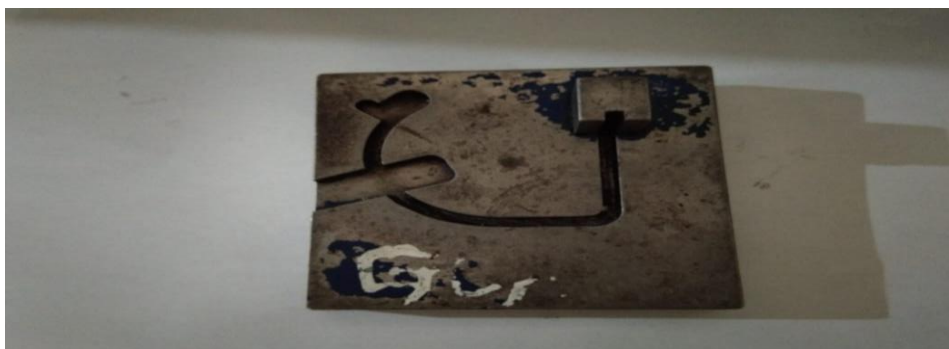
Gambar 4.13 Jig Inspection Guide Cable A
