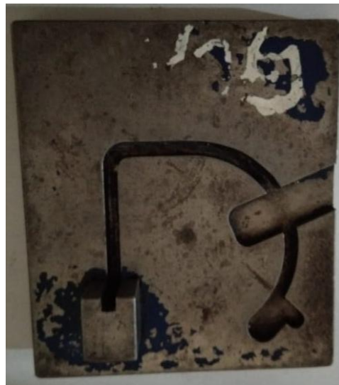
Gambar 4.5 Jig Inspection Guide Cable A
