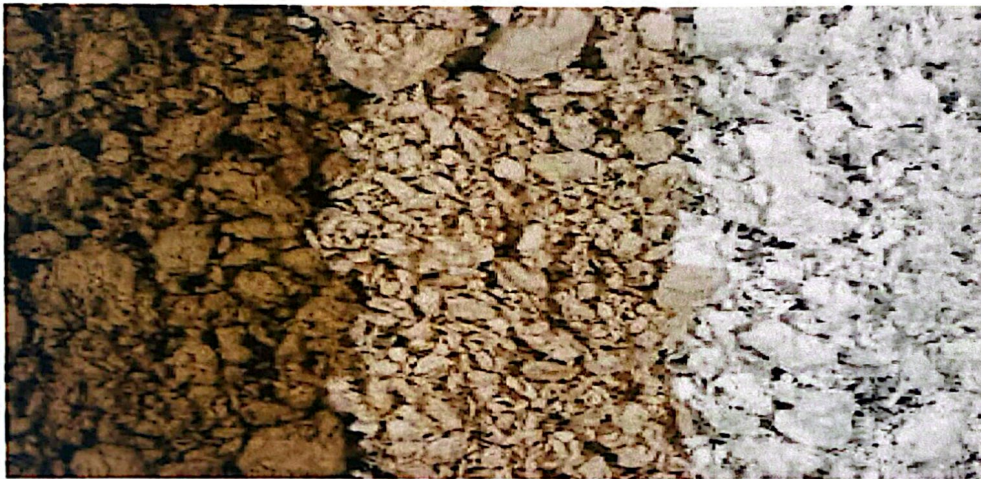
A B C Gambar II.4 Sampel bubur kayu setelah berbagai jenis proses kimia a) unbleached kraft ; b) unbleached sulfite ; c) bleached pulp (Banik dkk. 2010)
